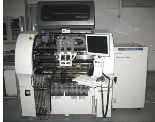
pick&place double head machine: Universal Genesis GC-60 (57000 cph)
