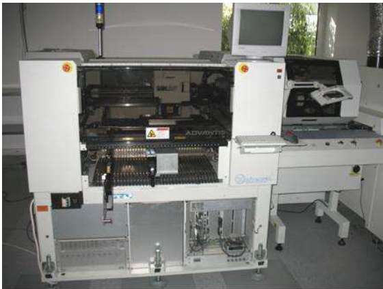
pick&place machine: Universal Advantis AC-72 (14000 cph) platform tray feeder Universal
